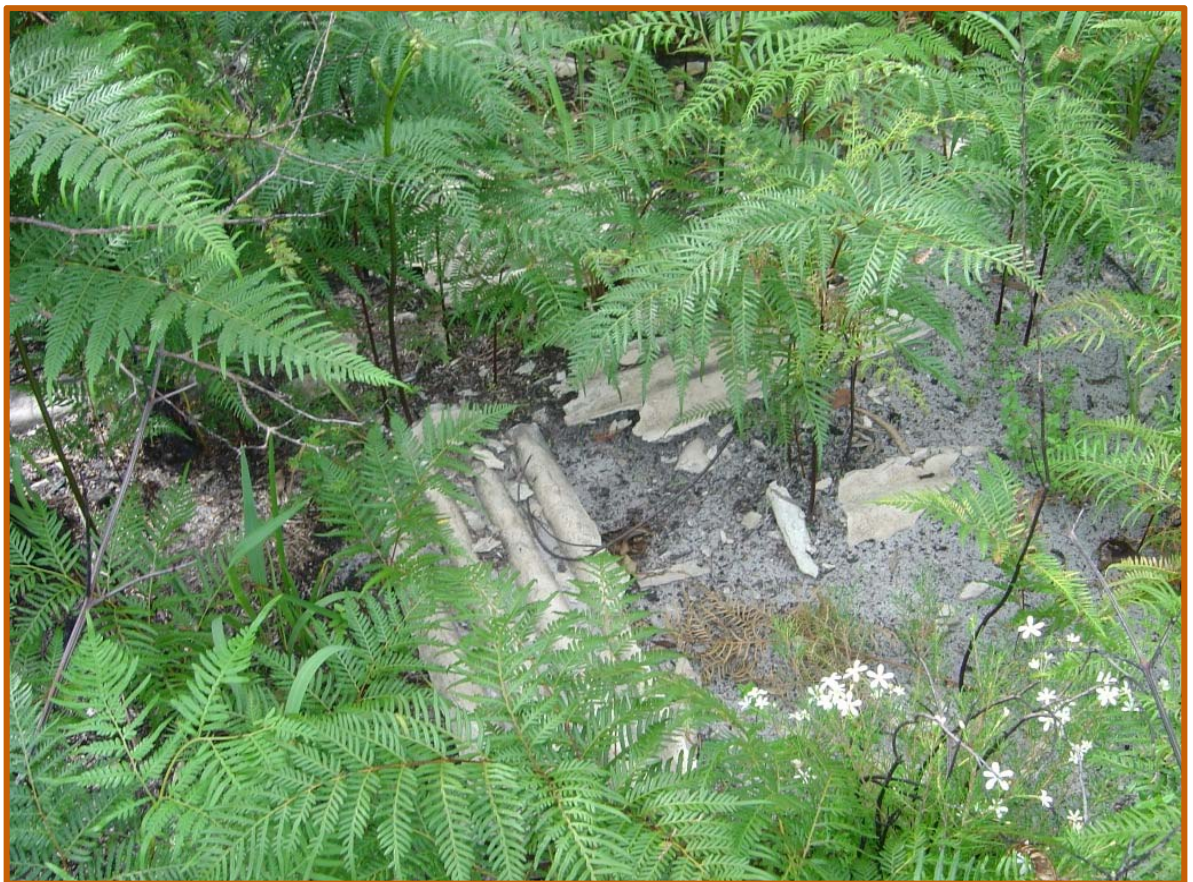
Photo 2: ACM sheeting - Previously encountered within the Northern Heavily Vegetated Area
